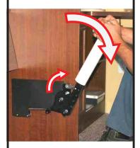
Sit on the ground and base your foot against the front edge of the side panel. Use a PVC tube and pull the arm towards you to free the silver blocking bracket. Ease the arm back slowly.
