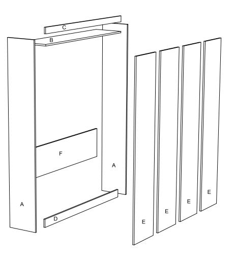
All dimensions are finished sizes All dimension units are in inches All material is 3/4 inch thickness
